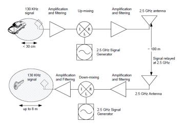
Figure 3: Up and Down Conversion and Modulation of Signal
