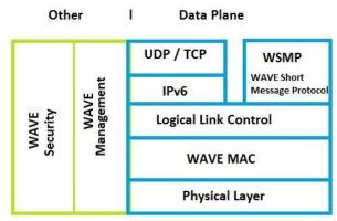
Figure 4. Wave Protocol Stack
