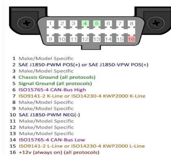
Figure 2. OBD2 Port as Data Link Connector
